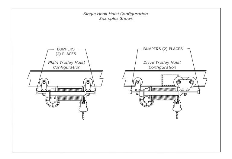
Neoprene bumpers reduce impact by absorbing energy when a moving hoist reaches the end of its permitted travel by contacting an end stop, or if two moving hoists come into contact with each other.
