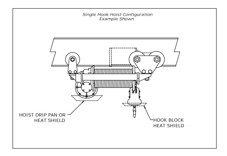
Drip pans reduce the amount of any foreign material falling from the hoist onto the work area below. Heat shields are used to protect the hoist and/or hook block in applications where high temperatures are present. Heat shields underneath the entire hoist are available. Contact Electrolift's Sale department for more information.
