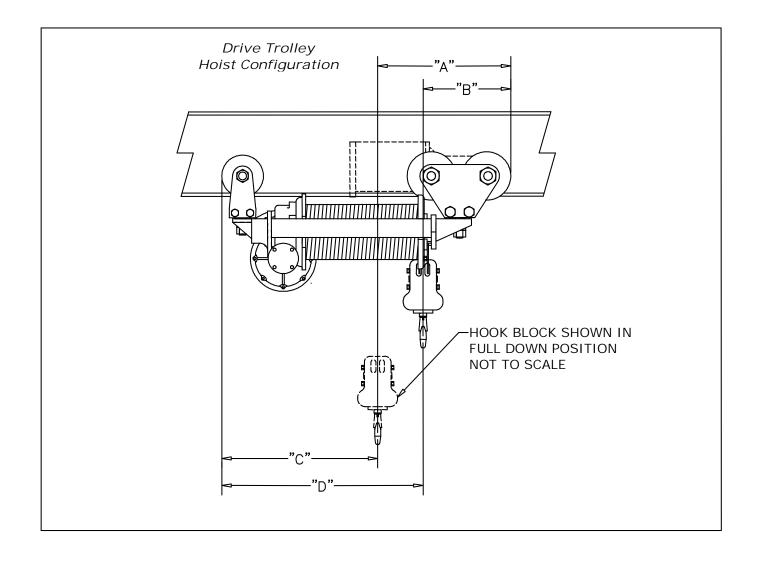
End Approach is the relationship between the hook and the outermost part of the hoist in the same axis as the track it is riding on. Depending upon the dimensional restrictions of a system, dimension "A", "B", "C" or "D" may be a limiting factor in hoist selection.
