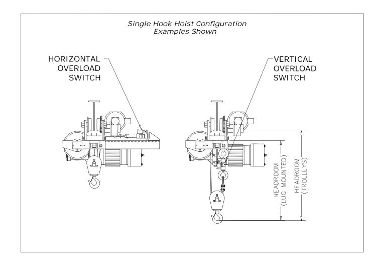
An overload switch will shut down the hoist up circuit when an overload condition exists. The switches are factory set to trip at a customer specified load level. The vertical configuration provides an economical solution where headroom loss is not an issue. The horizontal configuration provides overload protection without any loss of headroom.
