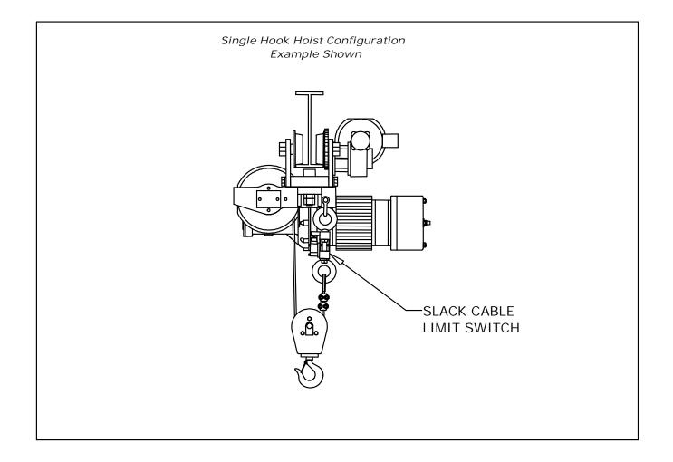
A slack cable limit switch will disable the hoist "down" control circuit when a slack cable situation exists. This feature is useful where limited visibility prohibits the operator from knowing when the load has been fully lowered. Twin hook hoists lowering devices in guides will detect a jammed condition when the wire rope goes slack. This will stop the hoist from continuing to lower the load. The load does not have the opportunity to dislodge itself from the jammed condition and free fall.
