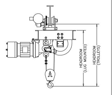
An overload switch will shut down the hoist up circuit when an overload condition exists. The switches are set to trip at a customer specified load level at the factory. The vertical configuration provides an economical solution where headroom loss is not an issue. The horizontal configuration provides overload protection without any loss of headroom.
