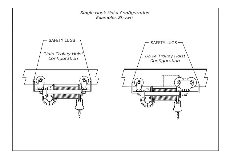
Safety lugs protect against any type of wheel, axle, or kingpin failure. The safety lugs engage the bottom flange of the beam and prevents the hoist from falling. Safety lugs are required by ANSI in all hot metal applications.
