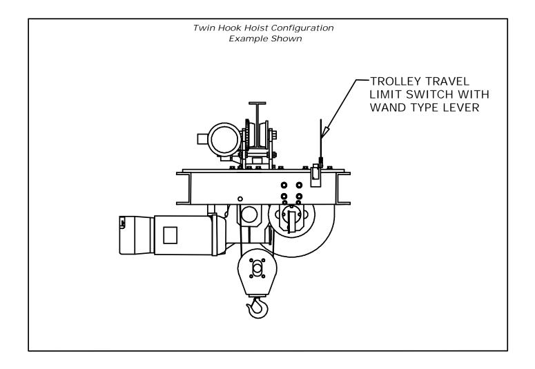
Trolley Travel Limit switches restrict the movement of a motorized trolley on a track. A wand type limit switch engages an end stop cam, and disables movement in the direction the cam was engaged. The location of the switch relative to the track must be agreed upon with Electrolift.
