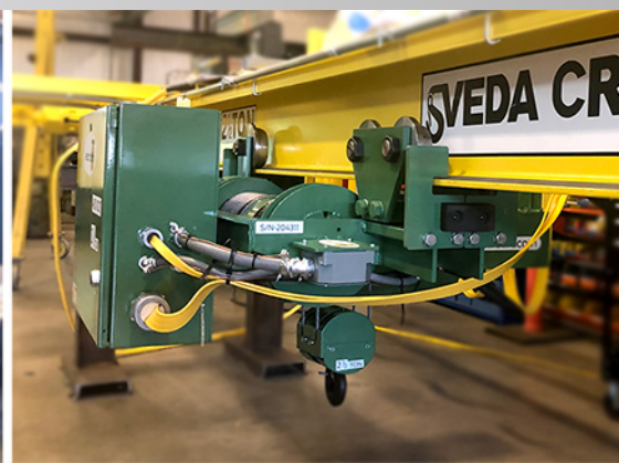
Left: True vertical lift and low headroom highlight Electrolift’s simple and effective design.
