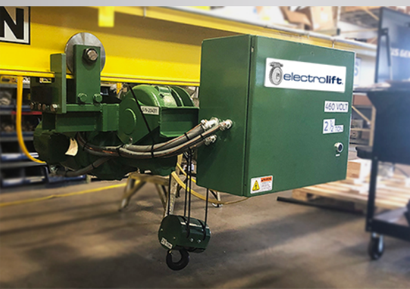
Left: True vertical lift and low headroom highlight Electrolift’s simple and effective design.
