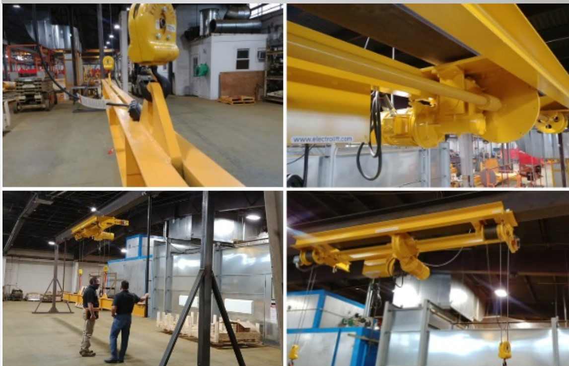
Top left: The centerpiece of the installation was a 1-ton capacity twin-hook Caldwell lifting beam. Top right: Electrolift designed a 2-ton capacity twin-hook hoist with a rigid (lug) mount to the beam. Bottom left: The system was assembled and tested onsite at HSI prior to shipment, including a load test. Bottom right: The system was completely designed from the ground up.
